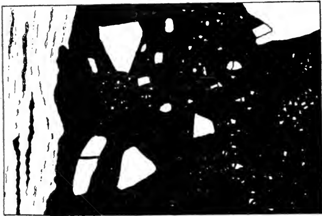
Fig. 14.—Character of ore at Levack mine, third level, Sudbury area, Ontario. Black represents sulphides; white represents granite-gneiss. Width of face 4 feet.
